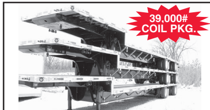
39,000# COIL PKG. (2) 2012 Utility 48'x102" Drop Deck Trailers, air ride, alum. floor, alum. comp., 39,000# coil pkg., 121" spread, 255/70R22.5 Mich. tires, 11,477 lbs., call!
