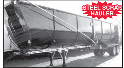
STEEL SCRAP HAULER 2012 MAC 44' Steel Frameless Scrap Hauler, AR 450 body, alum. draft arms, electric mesh tarp, air ride, 89 cubic yard, empty weight 19,400#, stk# 15724.
