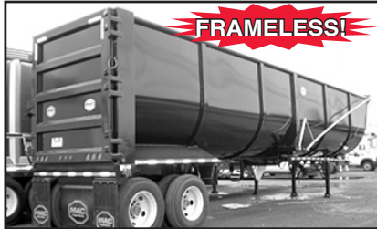
FRAMELESS! 2011 MAC 44' Steel Scrap Trailer (Frameless), 96" sides, Hardox 450, 89 cu.yd., air ride. In stock!
