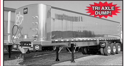
TRI AXLE DUMP! 2010 MAC Dump Trailer, 36'x102" w/66" sides, tri axle w/alum. frame, smooth side, alum. wheels, (2) way gate.
