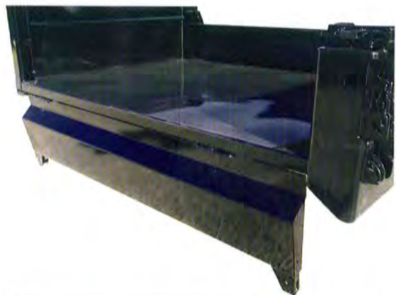
Pictured is a view of the 12' PLD drop side option. With the release of the two independent spring latches the side folds down below the floor. The 14' and 16' dropsides are split. (two sections each side)
