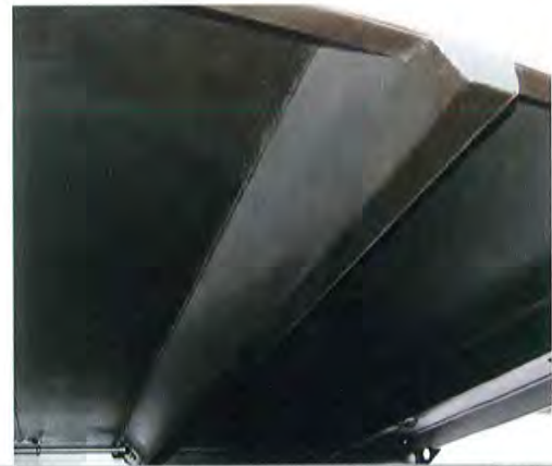
The crossmemberless understructure of the 130U & 133U Crossmemberless body uses 3/16" X 100K formed 5" trapezoidal longbeams.
