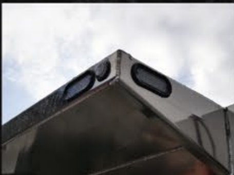
Strobe Lights in Cab Shield
