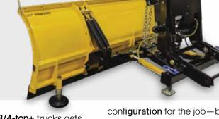
The Lot Pro for **3/4-ton+** trucks gets the job done fast with a **moldboard that stands 32" tall**, and an aggressive **75-degree attack angle** that also gives it superior back-dragging performance. Plus, it features **optional all-steel, multi-position wings** that give you the ability to choose the best configuration for the job—box, scoop or straight plow—by pulling a single pin.
