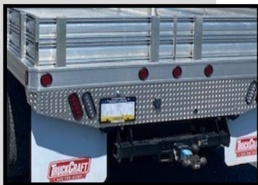
TAILBOARD 6" & 10" tall bright diamond plate wrap around corners includes license plate light and oval LED stop, tail, turn and backup lights.
