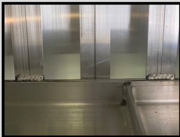
FLOOR CONSTRUCTION Plank extrusions provide rigid reinforcement every 5".
