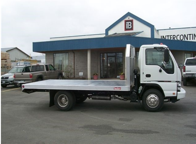
TC-500 MOUNTED ON A CAB OVER.
