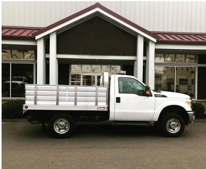
TC-500 MOUNTED ON A FORD PICKUP BOX DELETE WITH 24" RACK SIDES .
