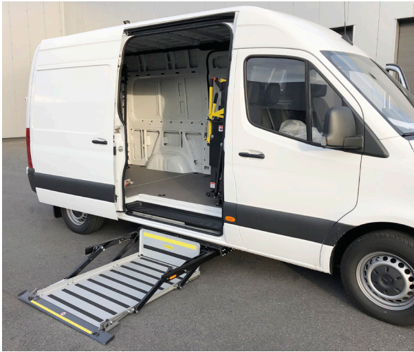
↑ DH-CH104.03 compact side mounted cassette lift • 650 lbs
