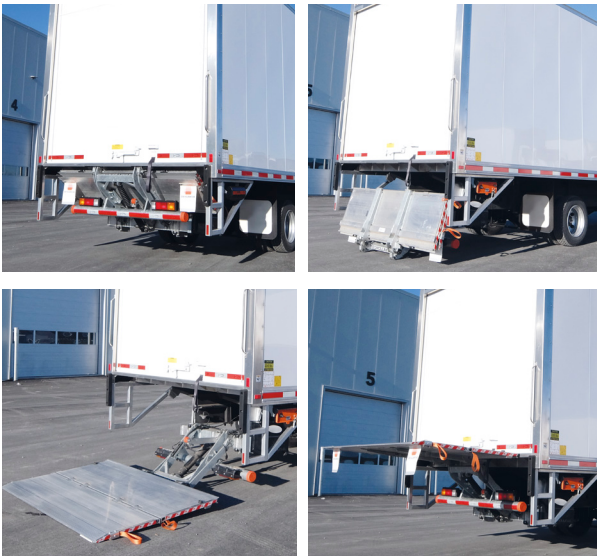
↕ DH-RPL light-duty fold-away liftgate • 1,650 / 2,200 lbs Narrow arm + 1 lift cylinder
