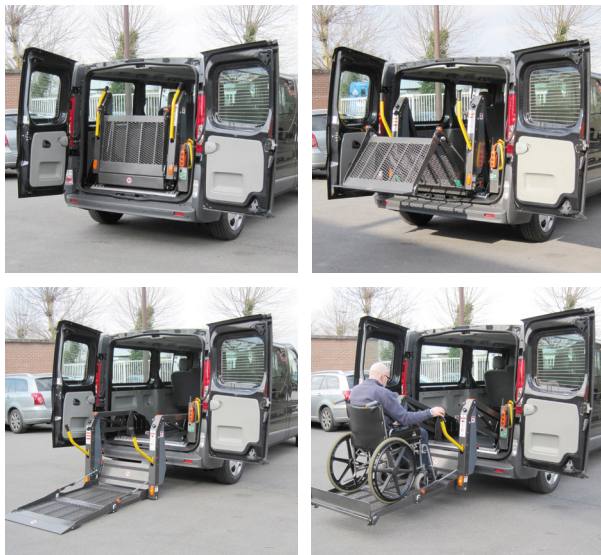
↕ DH-PH2.03 / DH-PH2.05 internal twin-arm lift with solid 1-piece platform, vertical split platform [OWU002] or horizontally folding platform [OWU003] • 770 / 1,100 lbs
