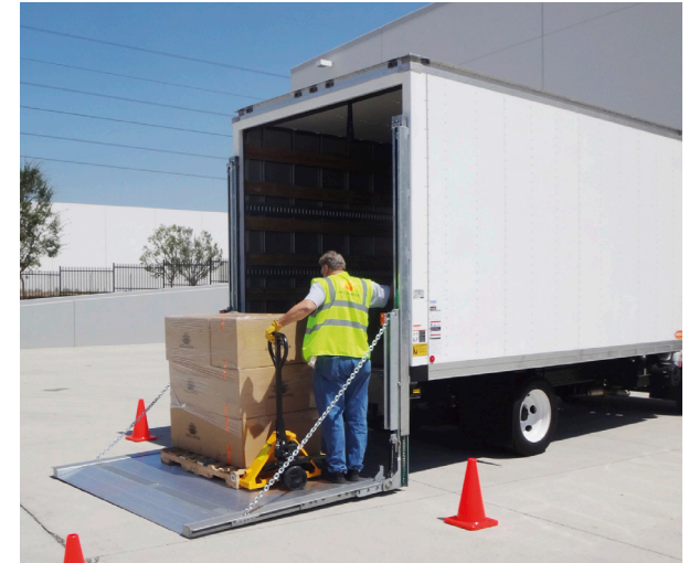
↑ DH-VOH.K9 column lift with long, chain supported platform, hydraulically opened and closed • 3,300 / 4,400 lbs
