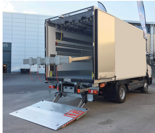
↑ DH-IV.10 lift for hanging meat • 2,200 lbs DH-SMM slider lift • 3,300 / 4,400 lbs
