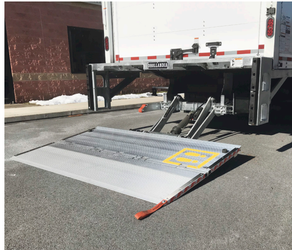
↑ DH-RPM medium-duty fold-away liftgate • 2,500 lbs Narrow arm + 1 lift cylinder
