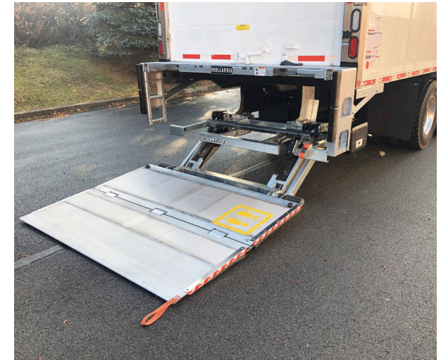
↑ DH-RMH extreme-duty fold-away liftgate • 4,400 / 5,500 lbs Wide arm + 2 lift cylinders • With bed extension
