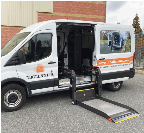
↕ DH-P2.04 / DH-P2.07 internal twin-arms lift • 1,100 - 1,650 lbs
