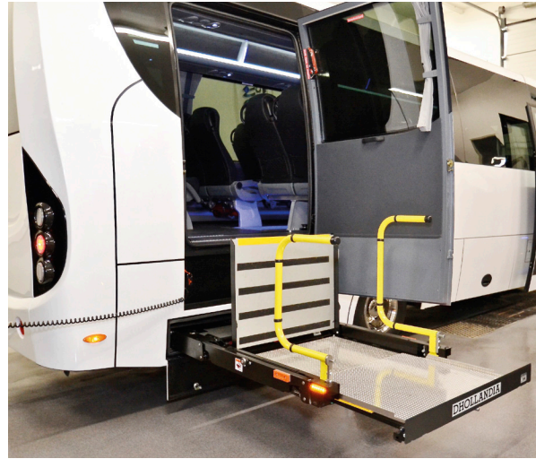
↑ DH-CH003.03 short cassette lift with extensible platform • 770 lbs
