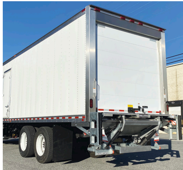
↕ DH-RMM heavy-duty fold-away liftgate • 2,500 / 3,300 / 4,400 lbs Wide arm + 2 lift cylinders
