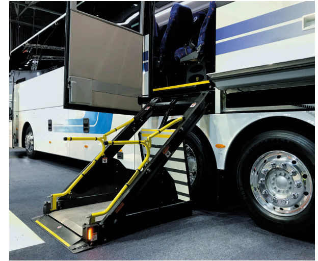
↑ DH-CH101.05 cassette lift with maximum travel downwards • 770 / 1,100 lbs
