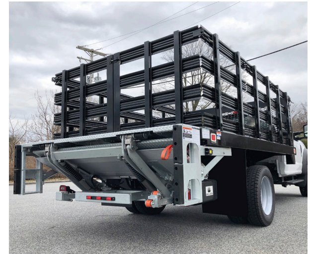
↕ DH-RPH heavy-duty fold-away liftgate • 2,500 / 3,300 lbs Wide arm + 2 lift cylinders
