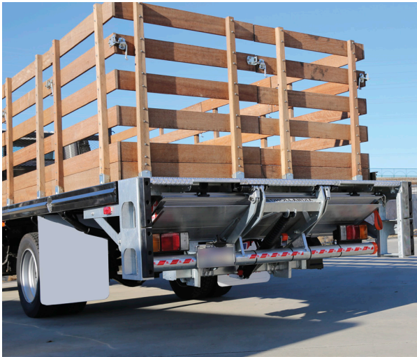
↕ DH-RPL light-duty fold-away liftgate • 1,650 / 2,200 lbs Narrow arm + 1 lift cylinder
