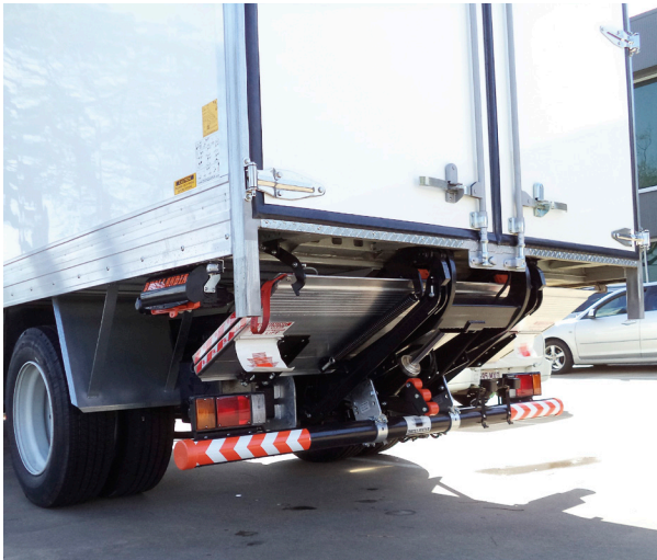
↑ DH-RCL light-duty fold-away liftgate • 1,100 / 2,200 lbs DH-RCM medium-duty fold-away lift • 2,200 / 3,300 lbs Narrow arm + 1 lift cylinder
