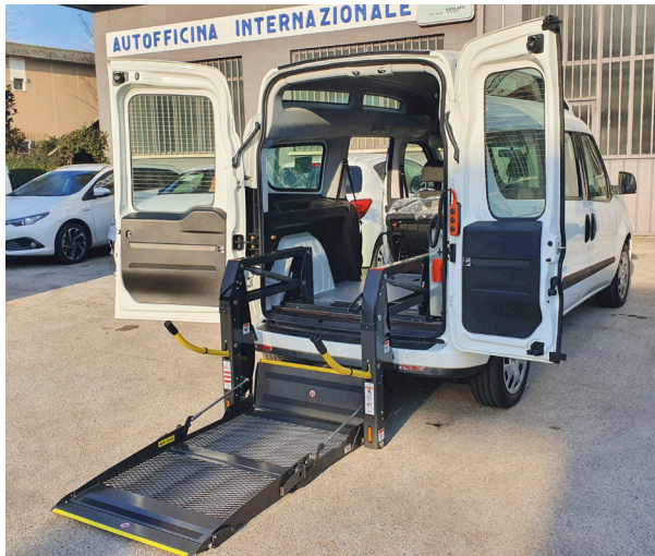
↕ DH-PH2.03 / DH-PH2.05 internal twin-arm lift with solid 1-piece platform, vertical split platform [OWU002] or horizontally folding platform [OWU003] • 770 / 1,100 lbs
