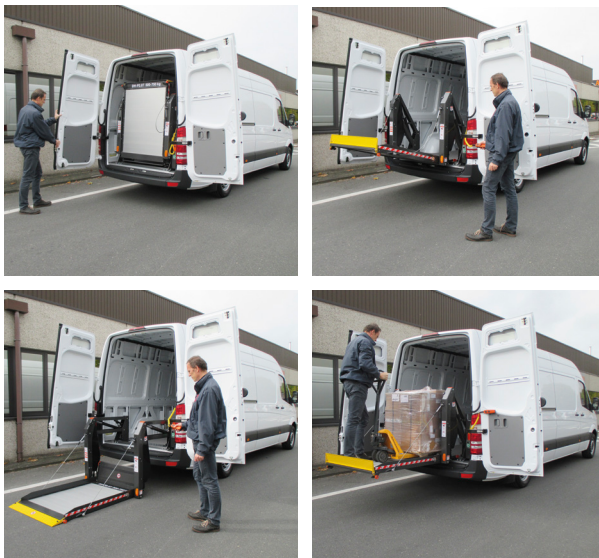
↕ DH-P2.04 / DH-P2.07 internal twin-arms lift • 1,100 - 1,650 lbs
