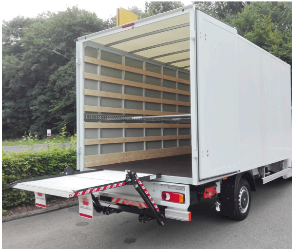
↑ DH-SC.05 City slider lift • 850 / 1,100 lbs
